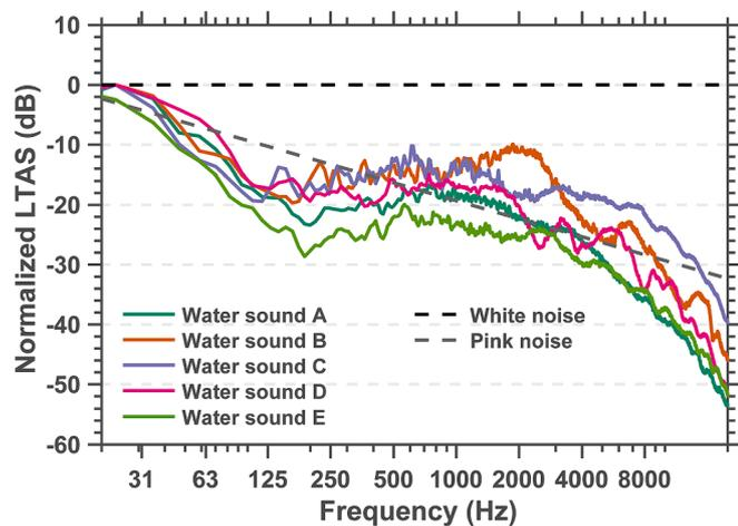
Fig. 2. Normalized long-time average spectral (LTAS) of five typical water sounds. Each LTAS was scaled with its maximum value. The black and gray dashed lines represent the theoretical spectral envelopes of white and pink noise, respectively.
