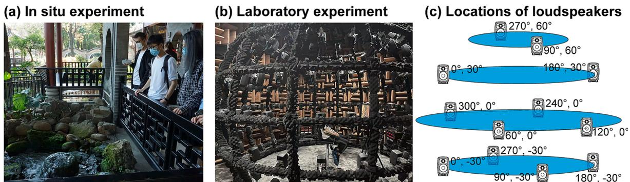
Fig. 4. Photographs of the in situ (a) and laboratory (b) experiments. (c) The spatial distribution of the loudspeakers for Ambisonics reproduction. The coordinate of each loudspeaker position is marked as  $(\theta, \varphi)$ , where  $\theta$  and  $\varphi$  denote azimuth and elevation, respectively.
